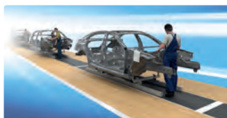
The Skid Transfer System
