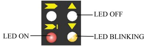
The operator can evaluate the main causes of the system stopping or failure using the 7-segment display and LEDs used to visualise the functions.
