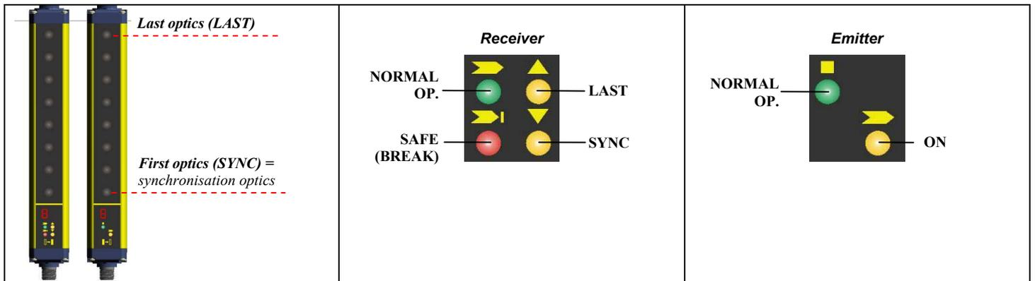
Signals are clearly identified through symbols allowing immediate reading, independent of bars directions. A short description of the signalling LEDs is necessary to avoid misunderstandings.
