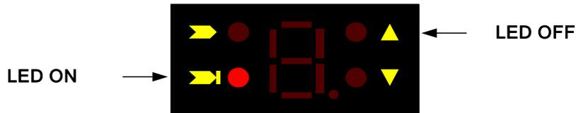
The operator can evaluate the main causes of the system stopping or failure using the 7-segment display and LEDs used to visualise the functions. For the receiver:
