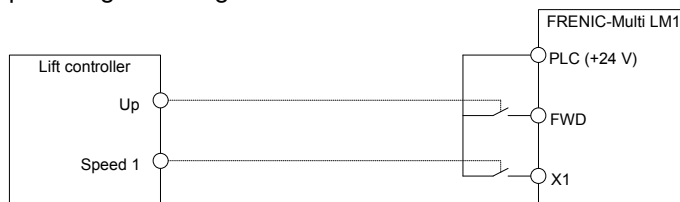
Figure 4.8: Normal connection using free potential contacts of the lift controller.
