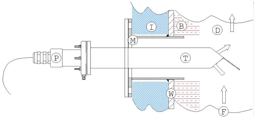
If the mating flange is mounted inside the insulation layer or even on the furnace wall, the accessibility for maintenance operation may be difficult and the flange gasket may be damaged by excessive heat.
