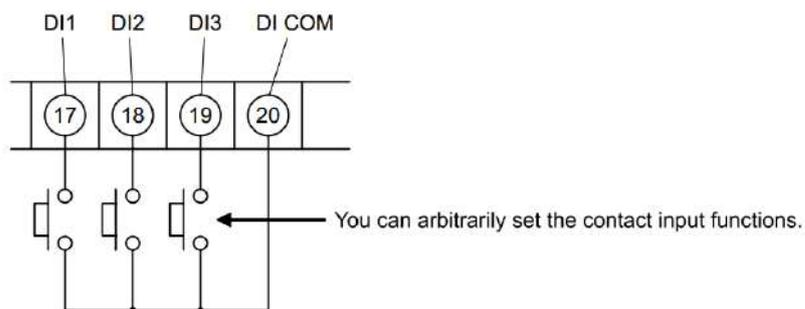
You can arbitrarily set the contact inputs (17), (18), (19) and (20) of the external terminal block. Piping and wiring for the standard gas cylinder and the solenoid valve shall be installed.
