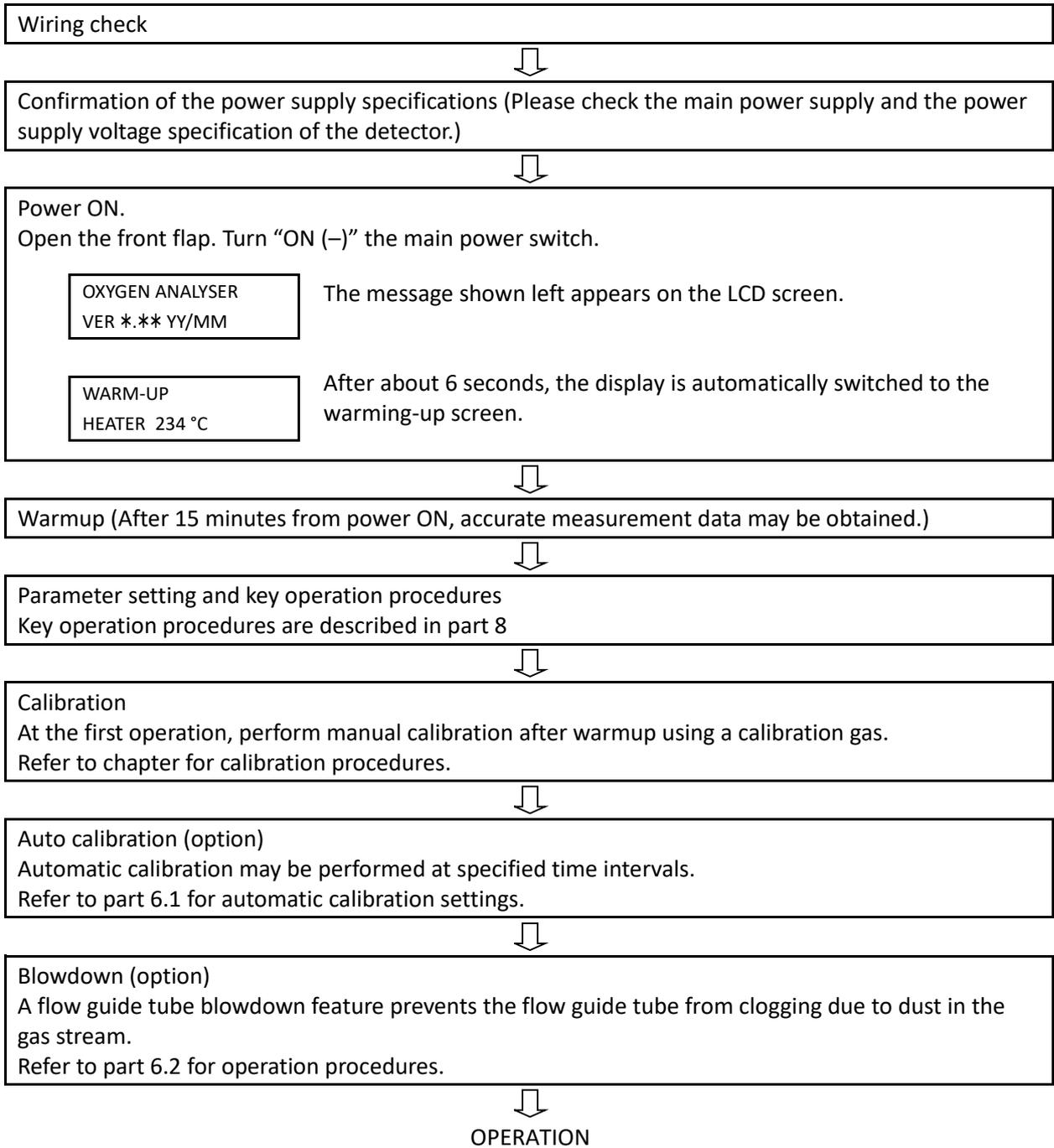
By turning the power on after completed piping and wiring, the transmitter turns on and the probe warm-up starts. The sensor usually takes approximately 30 minutes to reach the operation temperature which is 800°C for O2 probes.
