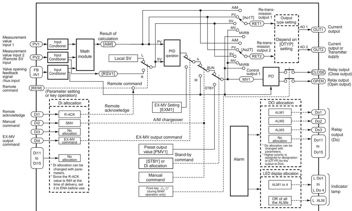
\* Valve opening feedback input is used for the type of 5th digit "D" in CODE SYMBOLS.
