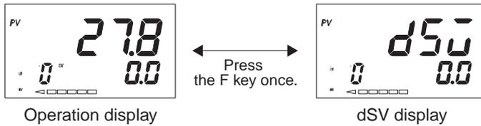
Note: Switching between the operation display and the dSV display can be done both in Auto and Remote operation modes.
