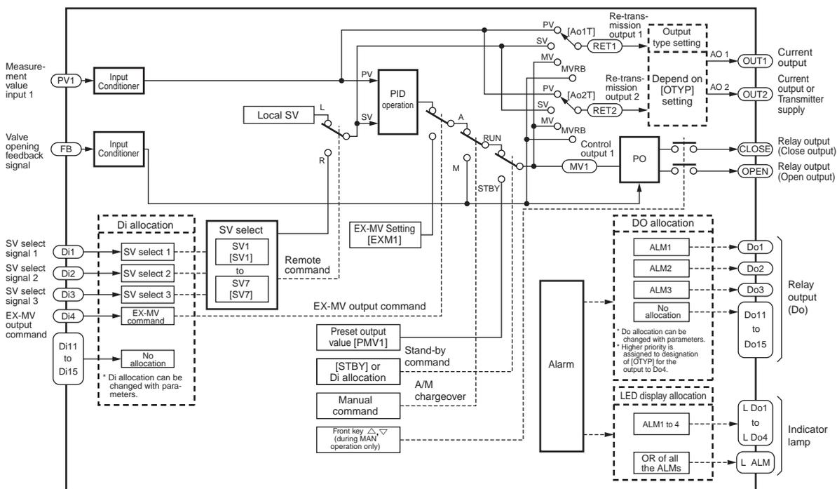
\* Valve opening feedback input is used for the type of 5th digit "D" in CODE SYMBOLS.
