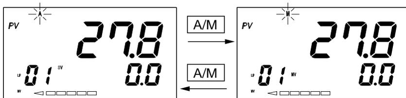
Related functions: [1] Prohibition of change to manual operation: Change to manual operation can be prohibited with A-M1 (Ch9-15) parameter. (See section 5-17 “Manual operation prohibition” for details.)
