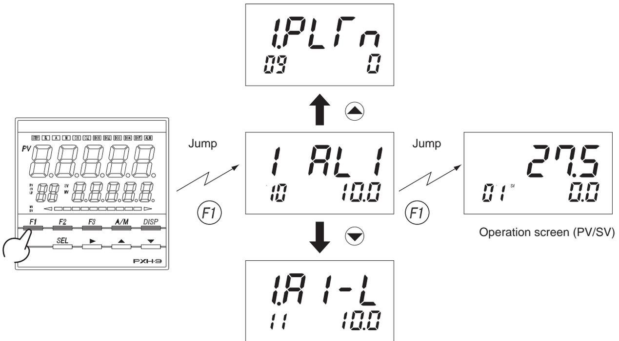
\* After a jump is made, transfer between parameters and setting can be made as usual.
