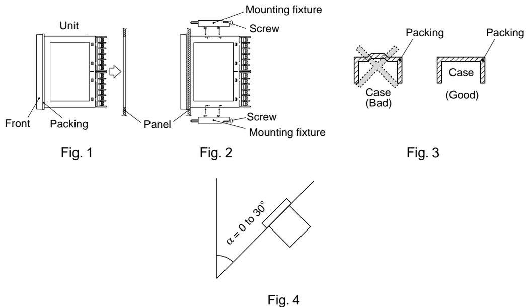
Standard: vertical panel attachment (horizontal position installing)
