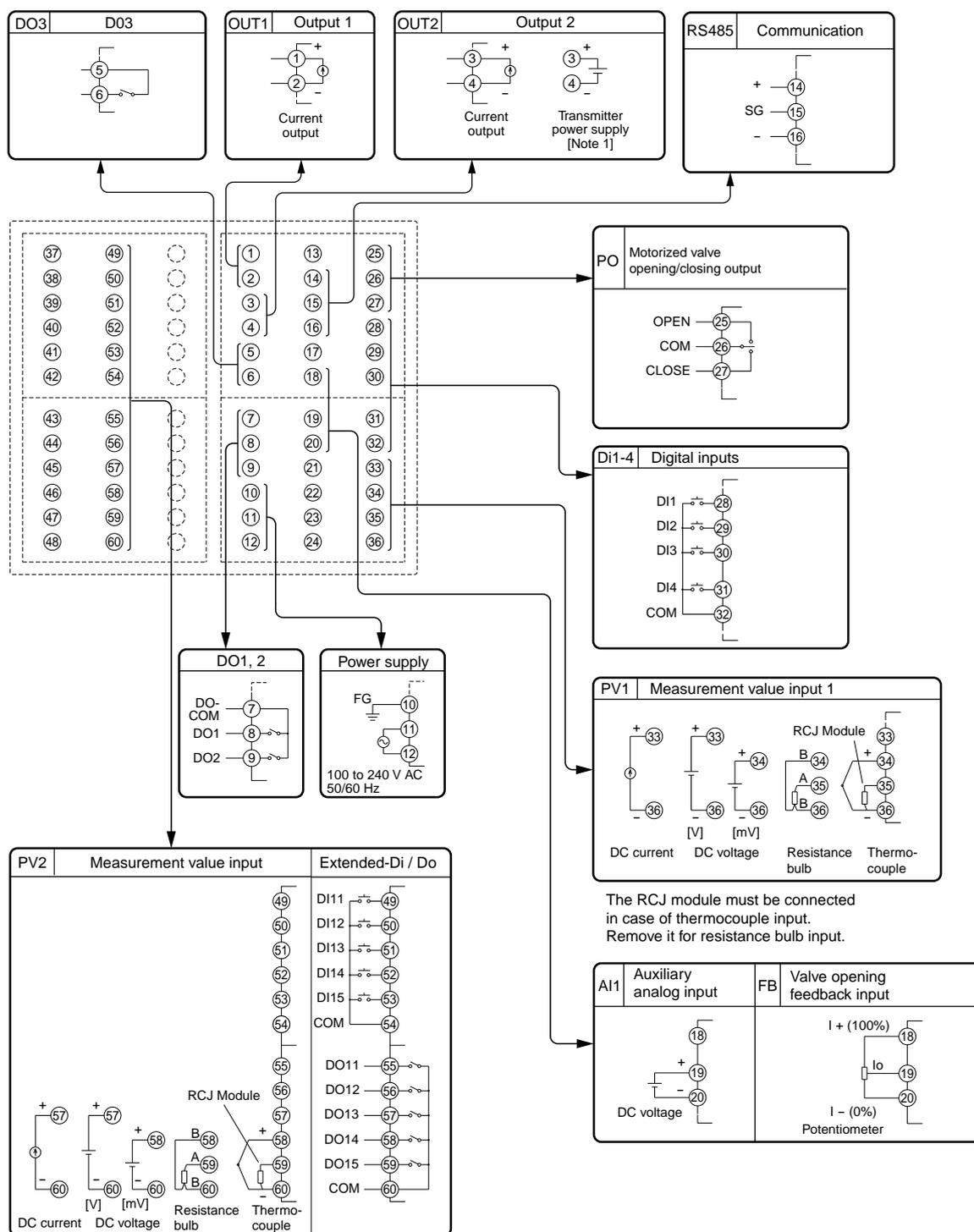
The RCJ module must be connected in case of thermocouple input. Remove it for resistance bulb input.
