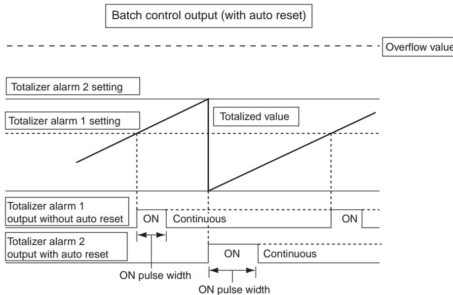
Note: The error of pulse width falls within 0 to 50msec.
