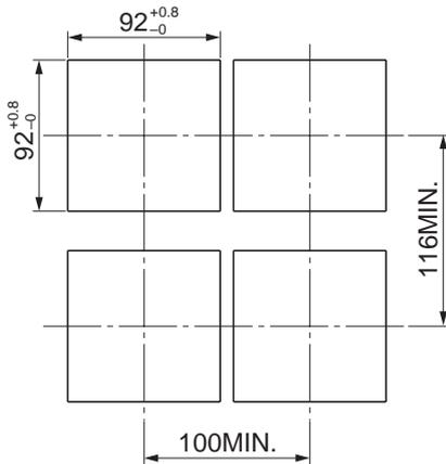
Note: In the case where a paint finish will be applied after panel hole-punching, take care of the finished dimensions.
