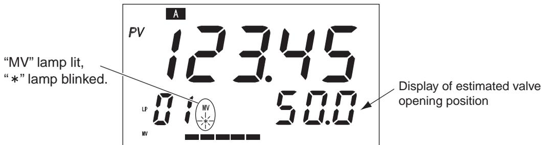
[Setting example] Changing the operation display type from 0 (MV) to 1 (MVRB)
